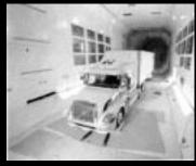
Results of testing published in SAE International 06CV-222 "Full Scale Wind Tunnel Tests of Production and Prototype, Second-Generation Aerodynamic Drag-Reducing Devices for Tractor Trailers"
