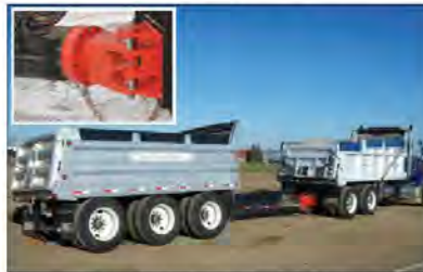
SAFER AND MORE PRODUCTIVE: A roll-coupling hitch design like this one (inset) allows for three extra tonnes of payload on tridem pony trailers in B.C.
