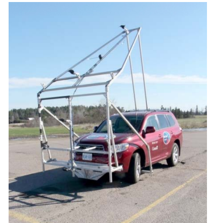
TC Test Vehicle instrumented by National Research Council (NRC) to gather on-road turbulence measurements.
