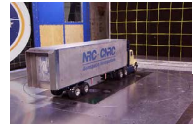
HDV model equipped with boat-tail in wind-tunnel.
