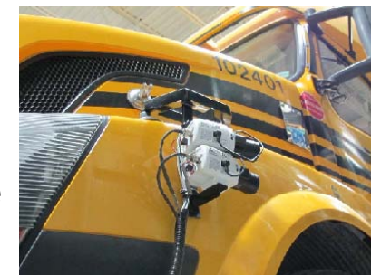
Prototype camera-mirror system equipped on Class VIII Vehicle.
