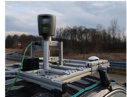
Vehicle equipped with 360 degree LiDAR system
