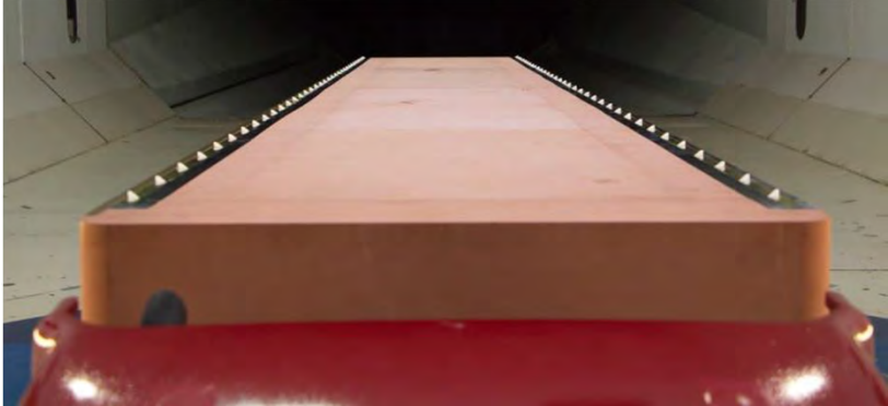
roof mounted vortex generators 34 per side
