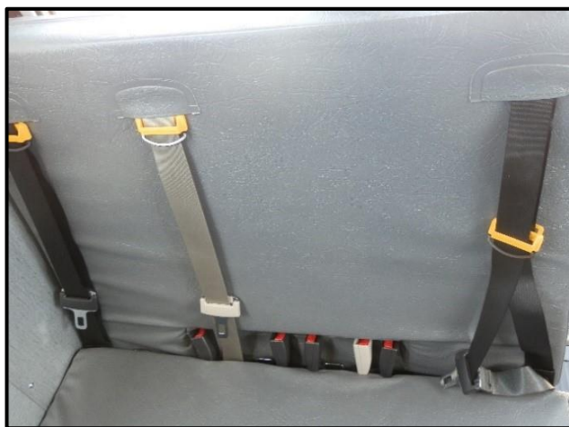
Figure 7. Example of coloured center seat belt and buckle (Not used on pilot buses)
