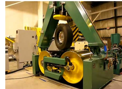
Rolling resistance and durability testing (Smithers Rapara)
