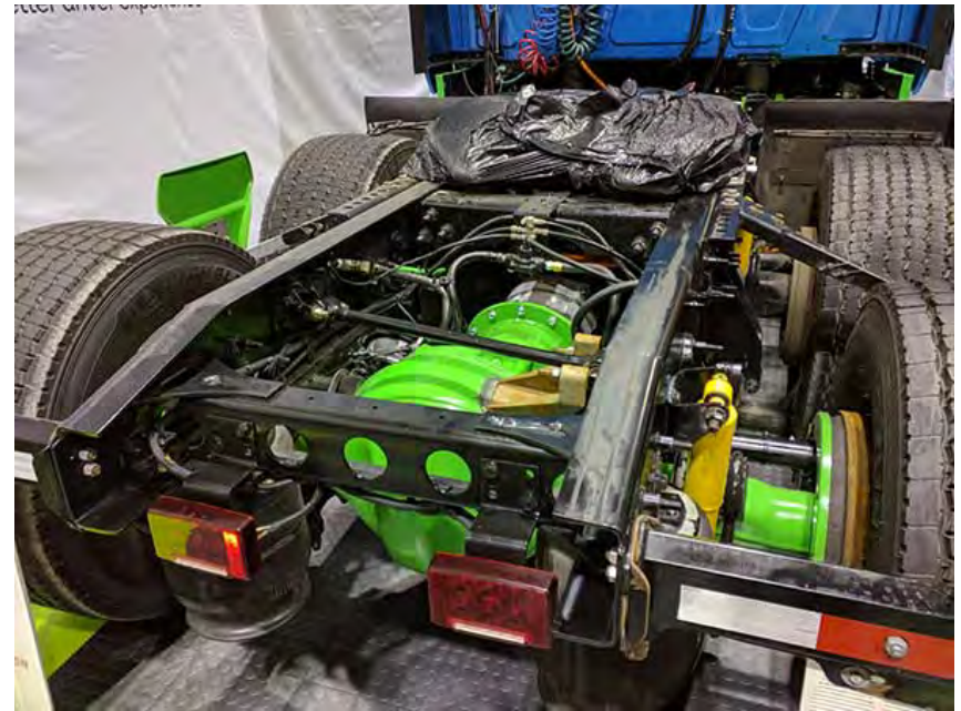
Hyllion 6X4HE Hybrid Electric System for Class 8 trucks
