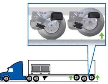
As the trailer load is reduced, the Meritor WABCO Trailer Lift Axle Control System will automatically raise the lift axle to reduce unnecessary tire wear and rolling resistance, thereby improving fuel economy and reducing costs.
