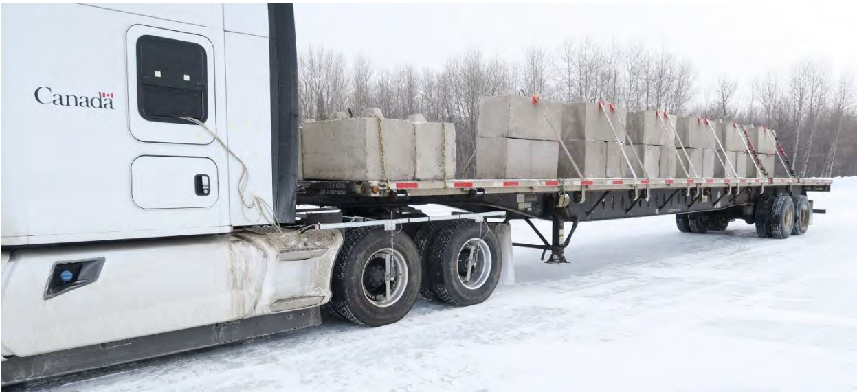
Figure 1: Ballast for Track Testing
