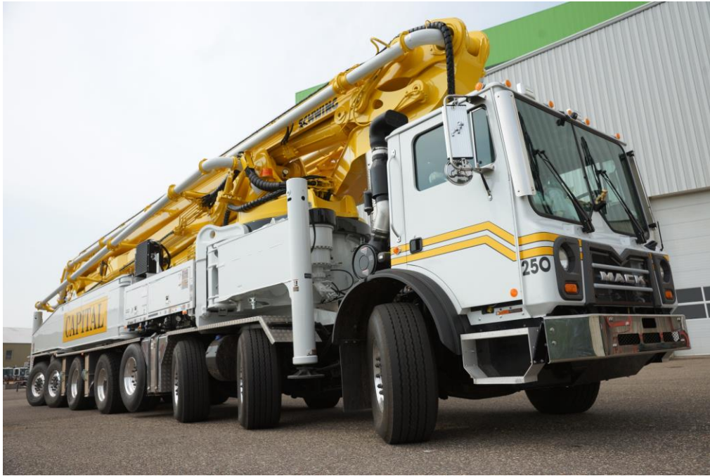
8 AXLE CONCRETE PUMP SCHWING AMERICA Tri-Steer – Lift (1) – Drive (2) – Steer Non-Drive; Drive steer
