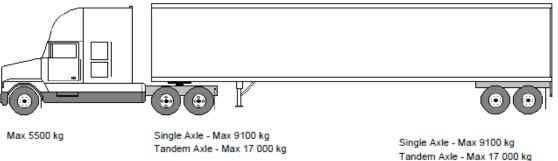
Tandem Axle - Max 17 000 kg Tridem Axle - Spread: 2.4 m to < 3.0 m - Max 21 000 kg 3.0 m to < 3.6 m - Max 23 000 kg 3.6 m to 3.7 m - Max 24 000 kg
