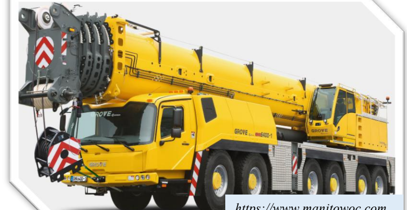
High-capacity 6 axle all-terrain crane – 400 tons
