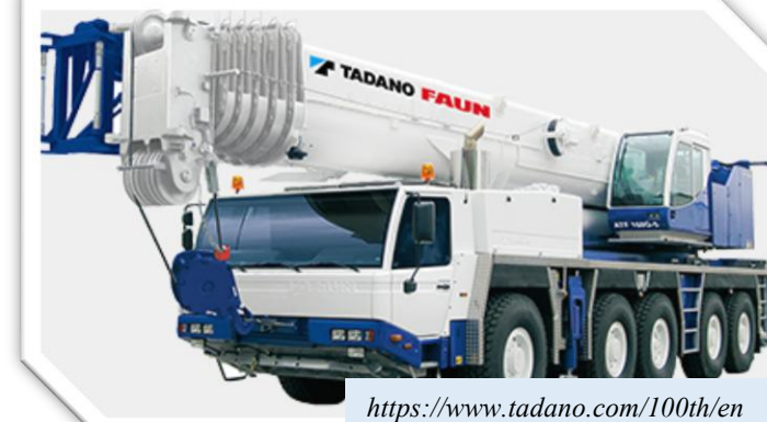
Mega-capacity 8 axle all-terrain crane – 550 tons
