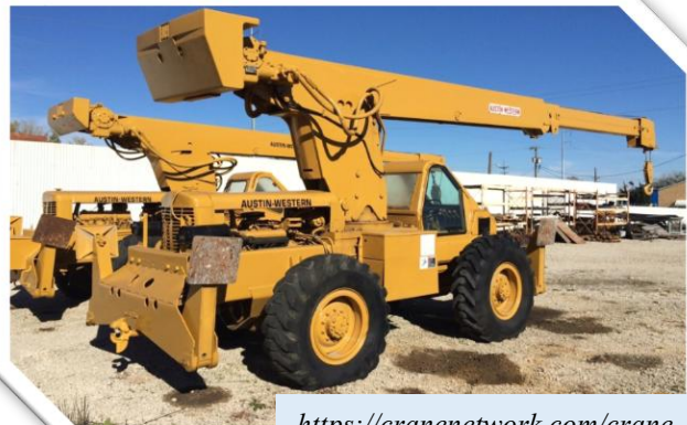
Early rough-terrain crane – 12 tons
