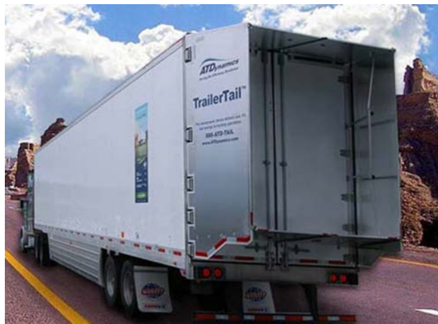
Figure 6. Aerodynamic side skirts and boat tails used to reduce aerodynamic drag (DOE, 2011).
