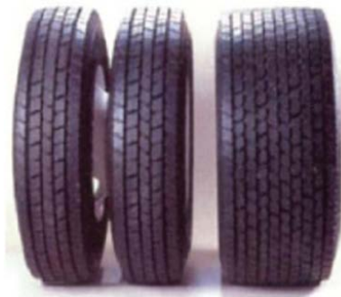
Figure 4. Comparison of dual tires and new generation wide-base single tires.
