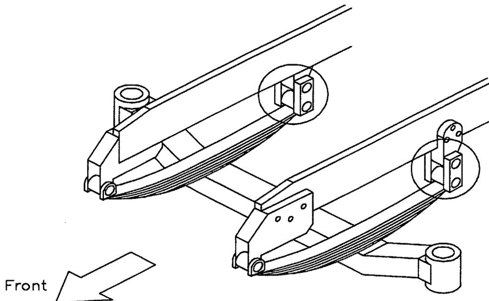
Figure 4. Location of instrumented shackles in front suspension.
