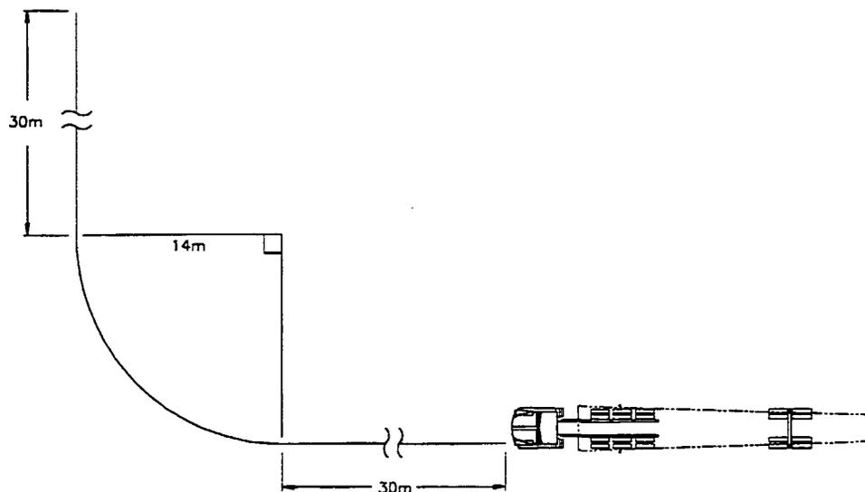
Figure 3. Steering response test path.
