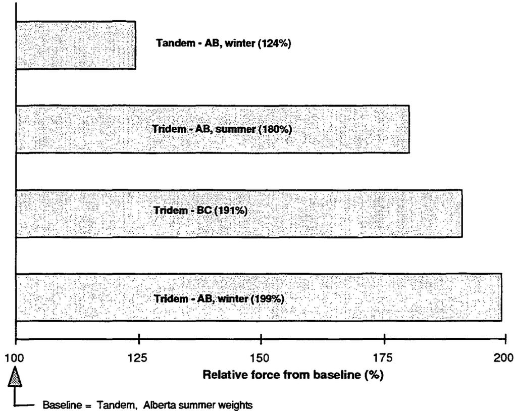
Figure 7. Peak force comparison: wet surface, no differentials locked.
