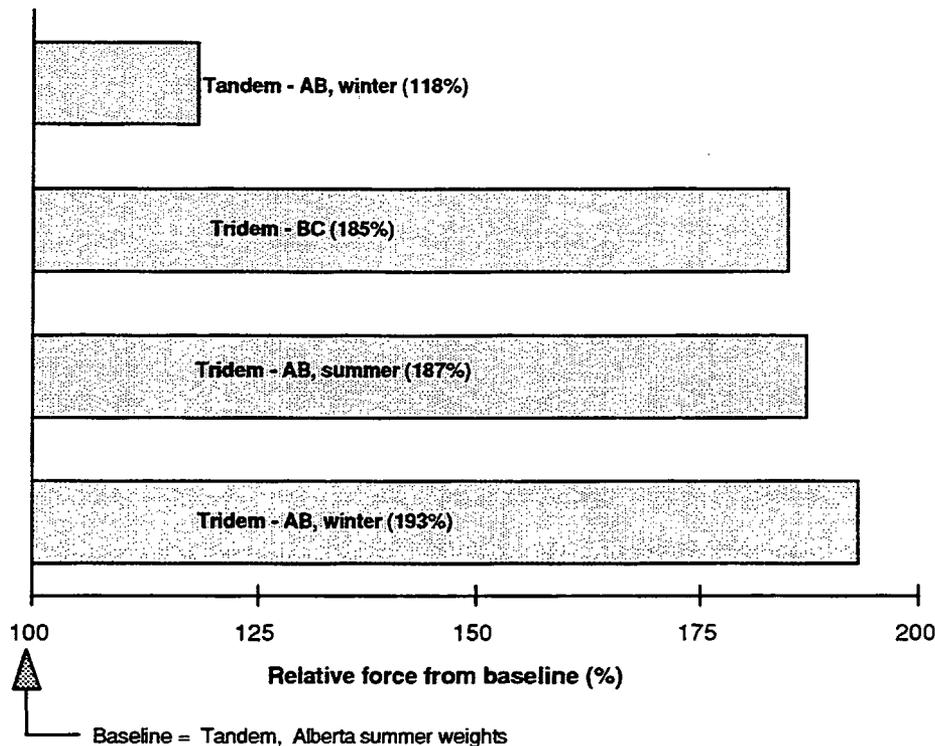
Figure 6. Peak force comparison: dry surface, no differentials locked.
